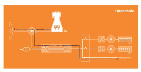
Island mode allows the entire electrical network to be created by the drive train.
