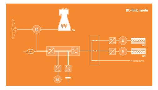
**DC link:** with the inclusion of a DC/DC converter and battery bank, the PTI mode can achieve a really advanced operational optimization. The DC link creates new possibilities for advanced ship design. The main switchboard can be smaller, and heavy users, such as big pumps, thrusters or battery banks, can be run more efficiently.
